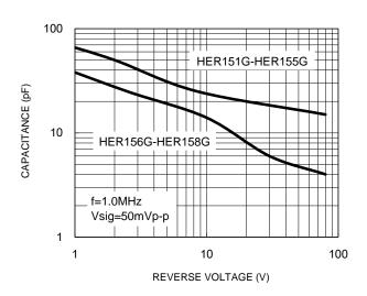
Fig.2 Typical Junction Capacitance
